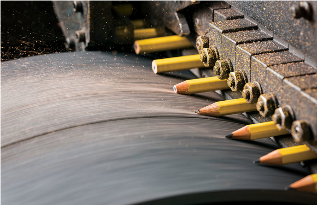
Pencils are sharpened on a high-speed sanding belt at General Pencil Company, Jersey City, New Jersey.
