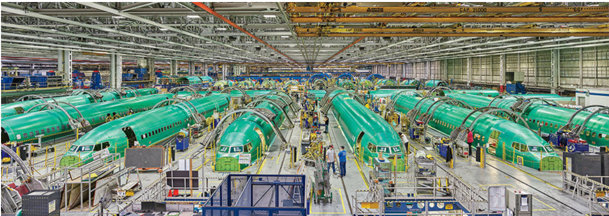
Workers assemble Boeing 737 Max fuselage sections at Spirit AeroSystems, Wichita, Kansas.
