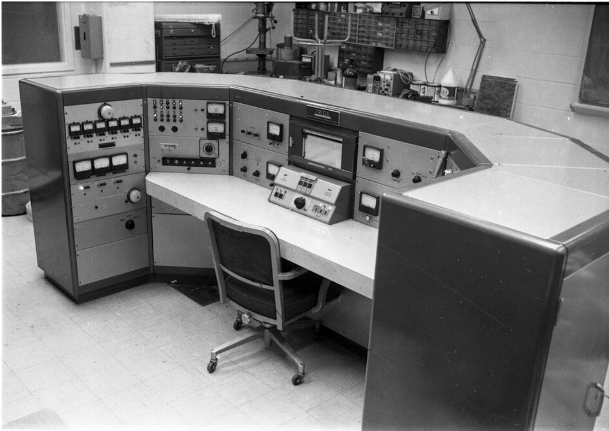
The control desk for the TRIGA II nuclear reactor in Mudd Hall. (Manny Warman / Office of Public Affairs / Columbia Archives)
