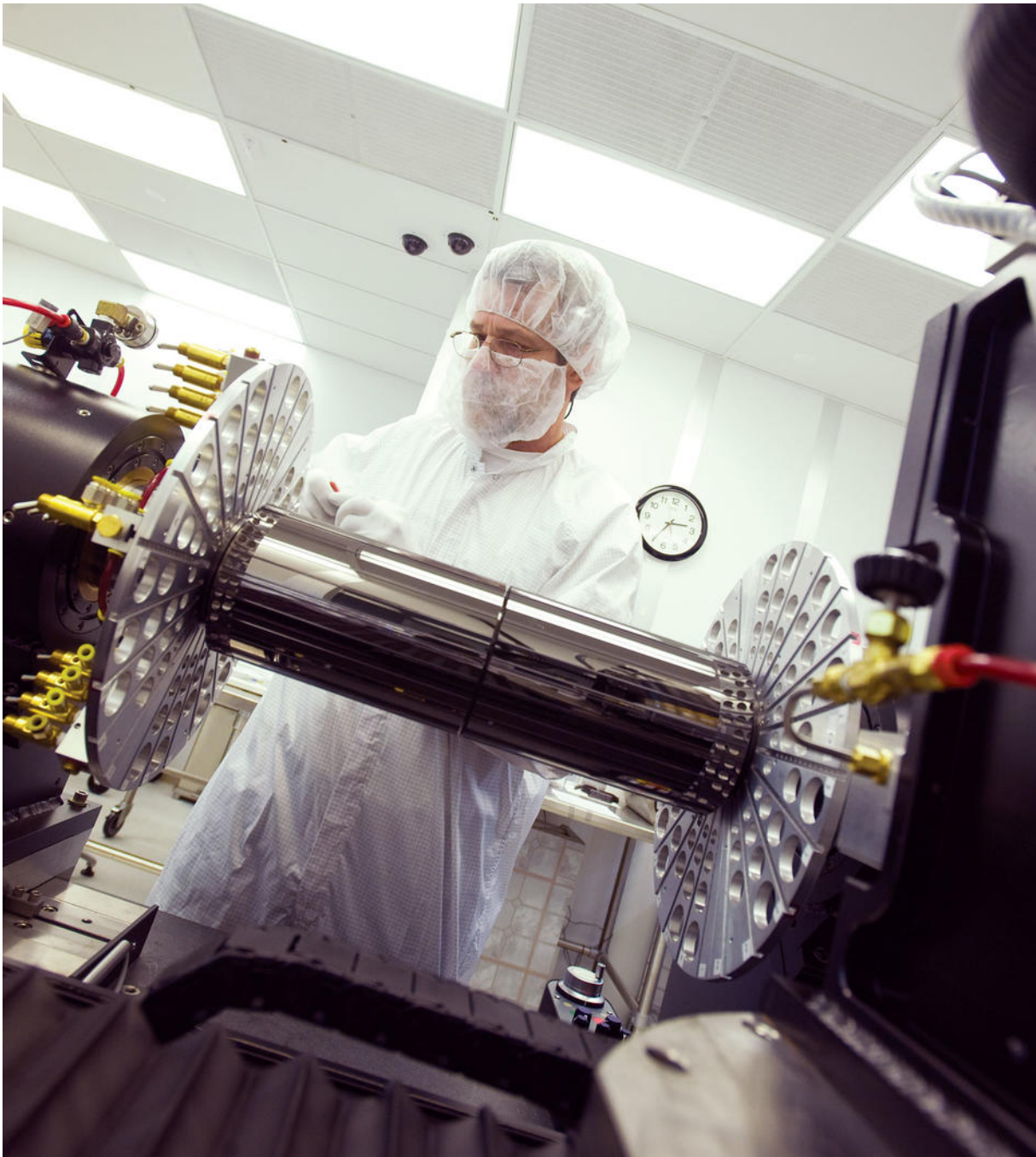
The optic device is assembled in a dust-free room, as any stray particles could hinder its performance. (Vernon Doucette)
