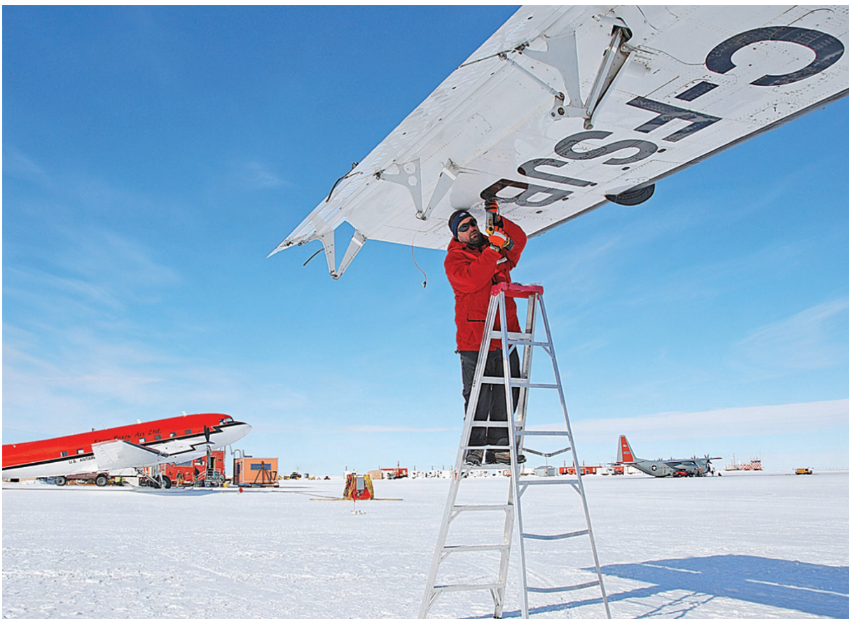
Michael Studinger opens an inspection hatch to connect magnetometer sensor cables to a computer inside the cabin. (Nick Frearson)
