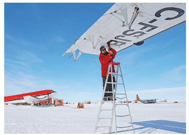
Michael Studinger opens an inspection hatch to connect magnetometer sensor cables to a computer inside the cabin. (Nick Frearson)
