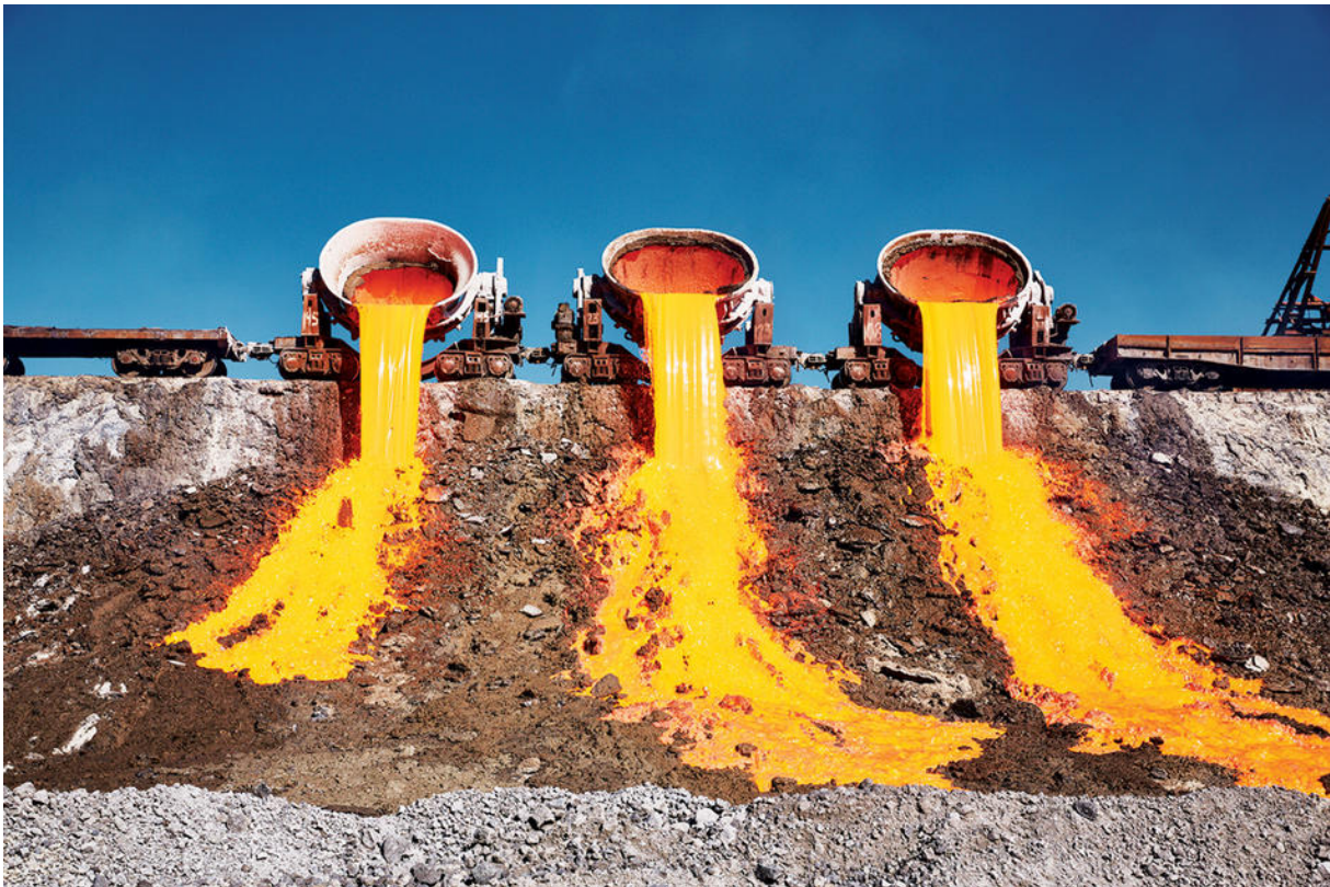
Molten slag is dumped into a landfill. Photo: Lenina11only / Shutterstock
