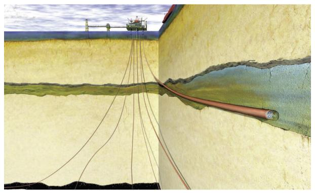
Columbia scientists say that vast amounts of liquefied carbon dioxide could be pumped underground or underwater into caverns made of basalt — hardened lava that reacts chemically with carbon dioxide to form a solid substance similar to chalk (Bug / Statoilhydro).
