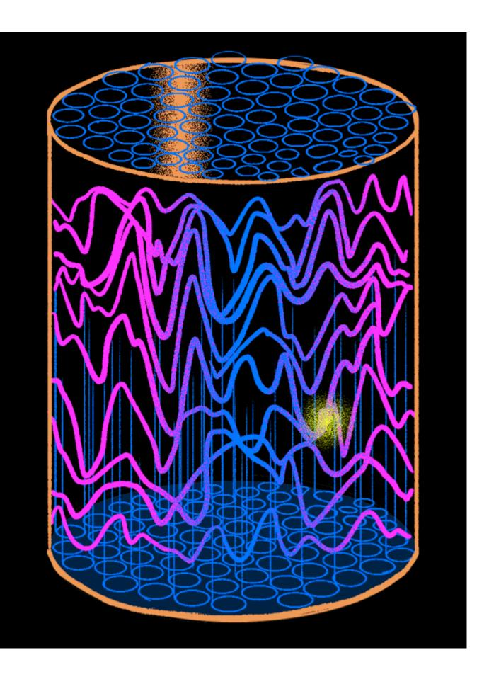
This would produce a minuscule flash of light — a pulse of energy so infinitesimal that 500 ultrasensitive photomultiplier tubes must be positioned atop and below the drum to detect it.
