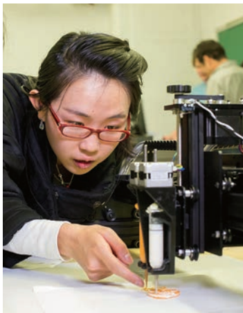
1. The printer's robotic arm can hold several food cartridges. This appetizer will be made out of goat-cheese polenta and beet purée.
