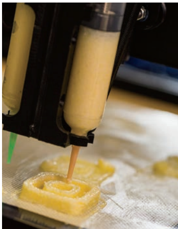
3. Multiple layers are extruded to create edible structures; the newest printer prototype can also cook the ingredients.
