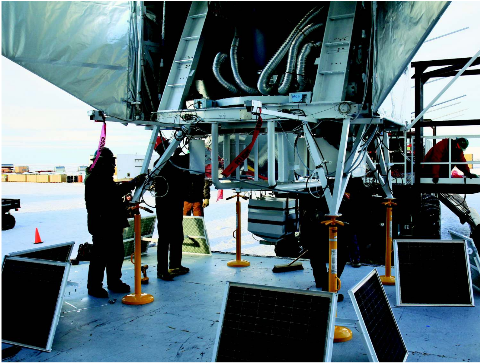
EARTH TO EBEX: (Above) Researchers conduct tests at the telescope's base to ensure that NASA instruments can speak to EBEX instruments. The dryer hoses near the top of the photo contain and protect data cables.
