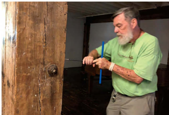
Edward Cook extracts a core from a beam in Manhattan's Terminal Warehouse.
