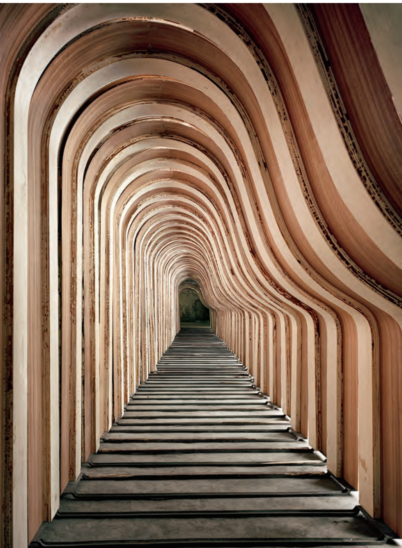
Piano rims sit in the rim-conditioning room at Steinway & Sons, Queens, New York.
