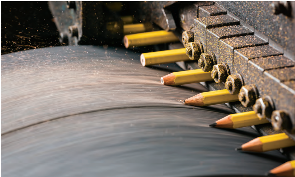
Pencils are sharpened on a high-speed sanding belt at General Pencil Company, Jersey City, New Jersey.
