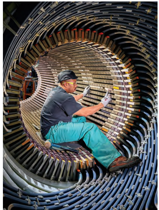
A hydrogen-cooled generator at GE Gas Power, Schenectady, New York.
